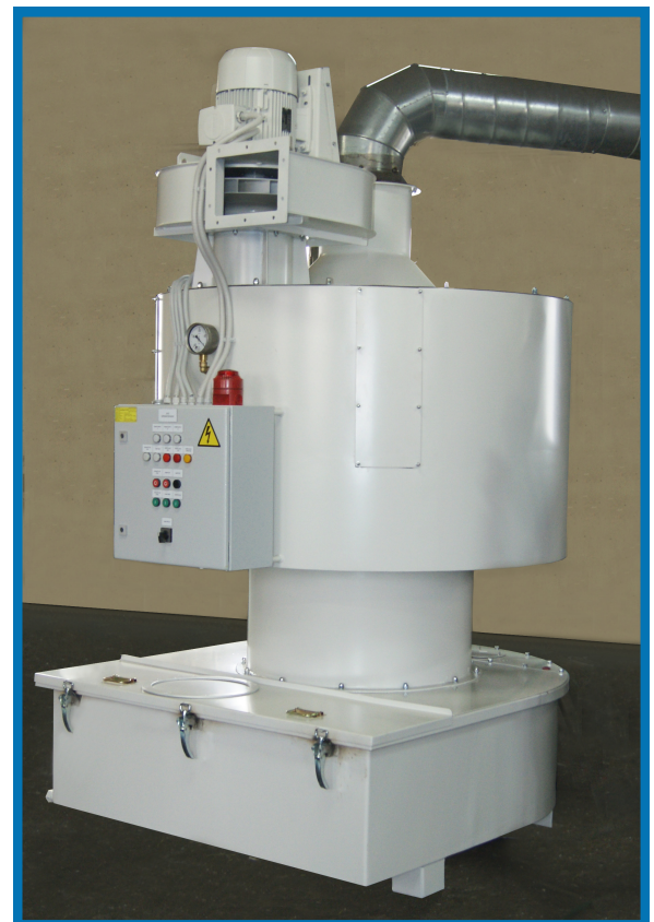
LGP-NÓVUM 4000 - made for the separation of flammable and explosive aluminum powder
